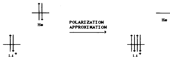
Figure 1. Unphysical transfer of electrons from He to Li + . It may occur in calculations that neglect the Pauli exclusion principle during deformation of interacting species. Actually, during deformation of the He monomer the occupied, low-lying 1s energy level of Li + is available for the electrons of He and the unphysical charge transfer takes place.
